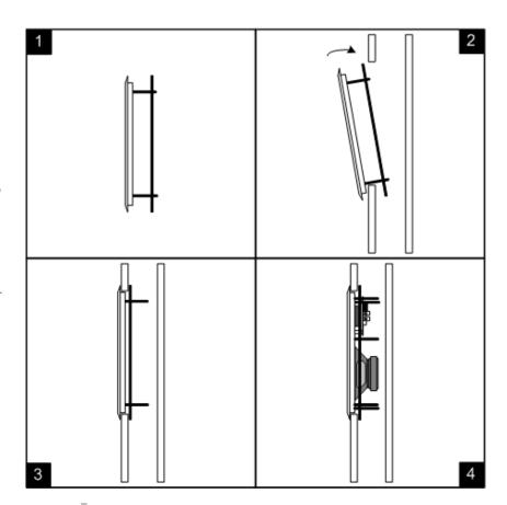
Once the frame is in place, gently tighten all of the screws so that the mounting ring is up against the back side of the wall board. (see fig. 3) Avoid over-tightening the screws or it may later become difficult to install the grille.
